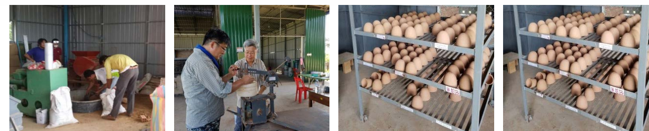
[Process of making Onggi filter: grinding, forming, formed cup shaped filter, firing]
